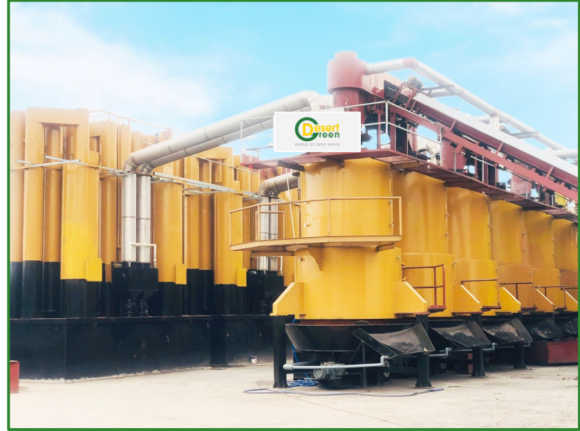
Section 2: RDF Gasification System of Linear Reactors
